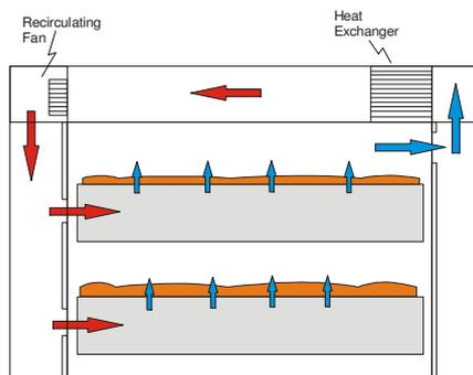
The problem is that each section needs to be separated from sections before and after so that air flow can be forced through the bed of product in that section. There is also a problem with ensuring the balance between 'make-up air' and 'exhaust air'. The ideal typical solution is shown below.
