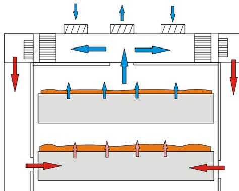
This diagram shows two recirculating fans in the section which then push air more evenly through the beds. The boxes at the top of the dryer show a central exhaust point with make-up air entering the air stream just before the two heat exchangers, the air then passing through the two recirculating fans before going through the product beds. Each of the sections needs to be separately balanced so that recirculating air temperature and velocity are optimised.
